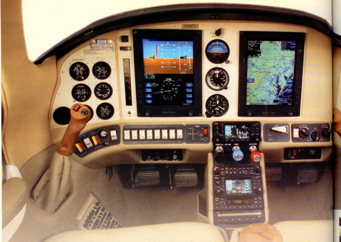
The pilot-friendly cockpit leaves plenty of room for new features later. The large, round wooden knob in the bottom center is the fuel selector.
